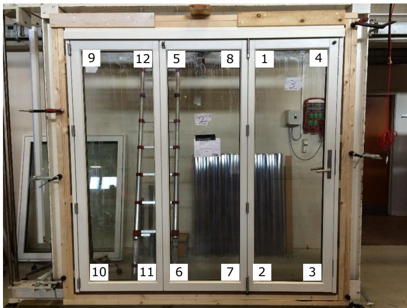
Figure 1: Static loading – Test sequence - Corner of infill
