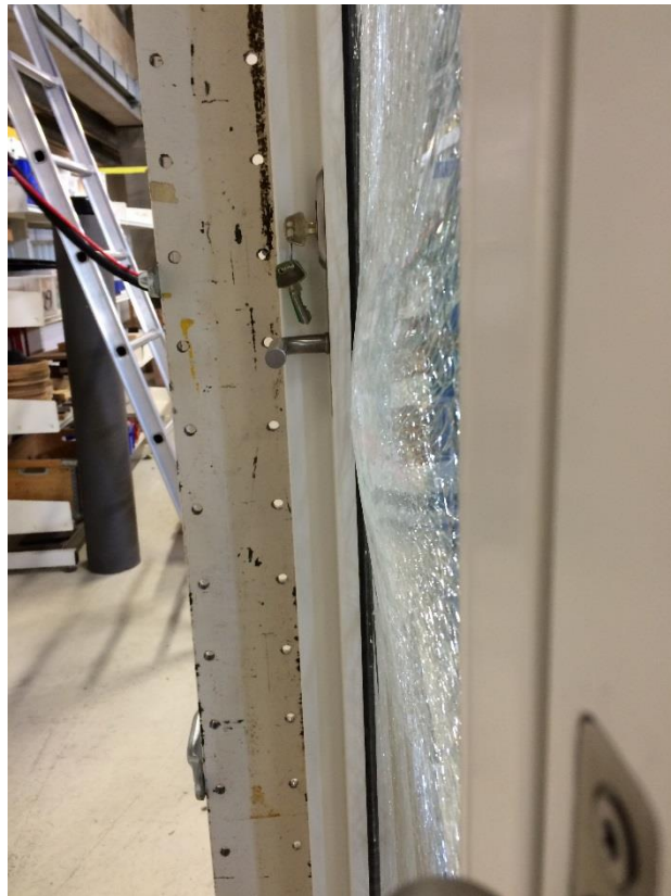
Figure 5: Glazing after dynamic loading
