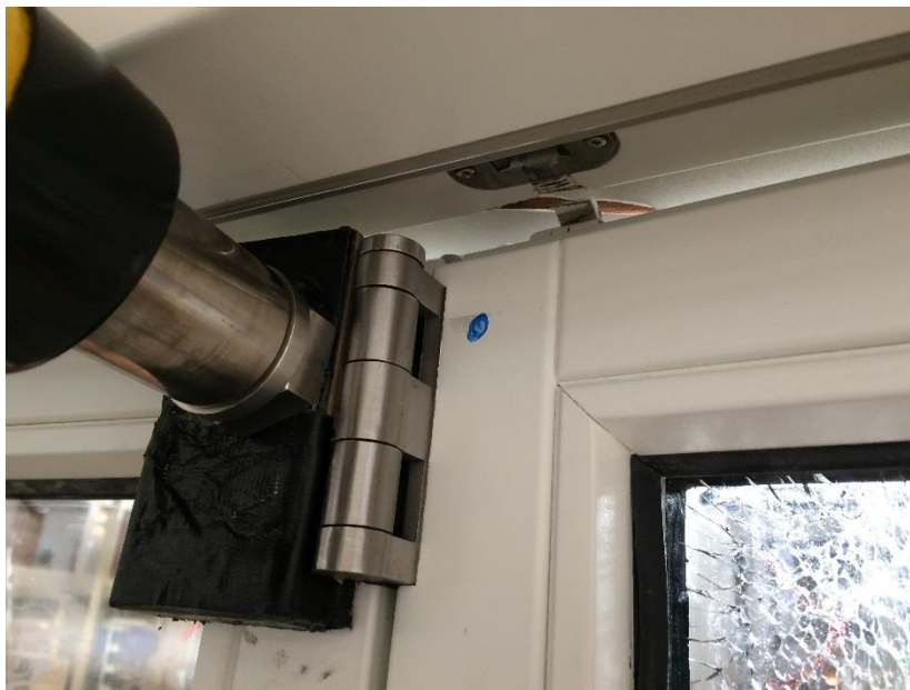
Figure 3: Locking point forced out during loading - not possible to pass gap gauge through opening
